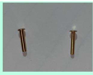
The 2009 version of the trolley pole pivot, part #12508 at left with the new 2021 version at right.
